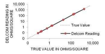
**REPEATABILITY**—Delcom meter readings are effectively 99.9% repeatable if sample placement and environmental factors, such as temperature, are held constant.
