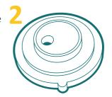
Tighten the screw in a manner that the disk can rotate smoothly with some slight friction. Light tightening is sufficient, don't overtighten.
