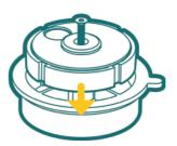
Insert the counter piece with screw Push counter piece, bottom and through the bottom and volume disk. Engage by aligning flattened indexing details of counter piece and top disk.
