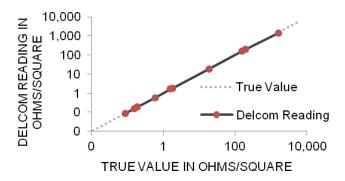
**REPEATABILITY**—The Delcom meter readings are effectively 99.9% repeatable if sample placement and environmental factors, such as temperature, are held constant.
